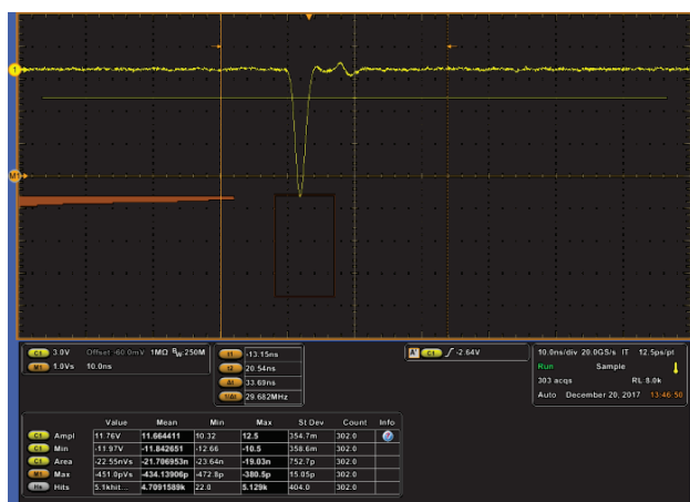
Fig. 3: Scope Charge measurement Q =300 pC FC in.
