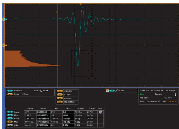
Fig. 4: Scope Charge measurement Q =33 pC FC out.
